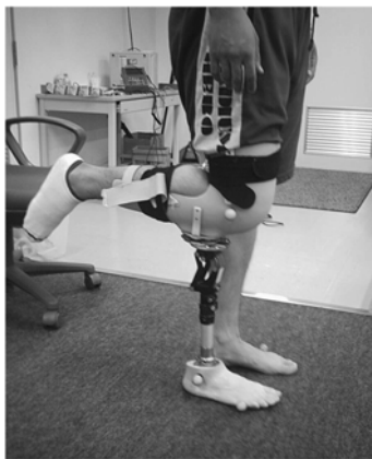
Fig. 2. Lateral view of the pseudo-prosthesis. Explain: Pseudo-prosthesis comprised a plate for maintaining knee flexion, a belt for immobilizing the upper and lower legs, a plate for adjusting the anteroposterior direction, a quadrilateral socket, and a single-axis joint foot.
